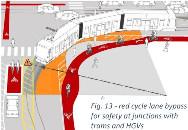
Fig. 13 - red cycle lane bypass for safety at junctions with trams and HGVs
